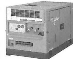
DIS-90SB 2.5m 3 /min 0.69Mpa
